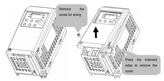
• The front cover is completely removed if lifting it up and removing the fixed part. Wiring and installation is available only with the cover removed.
