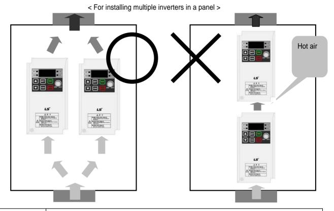
Arrange hot air from the inverters is discharged when installing them on a panel. 'X' shows incorrect layout example.
