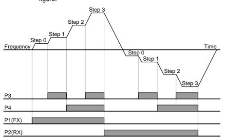
If running by using multi-step high/low, it is possible to run from 0 to 3 step in 4 combinations as the below figure.
