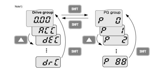
Can move between groups if pressing SHFT key in code 0 of Drive Group/PG Group as shown in the figure. If pressing SHFT in other codes but 0, it moves to the first code of a selected group and it moves between groups if pressing SHFT once more.
