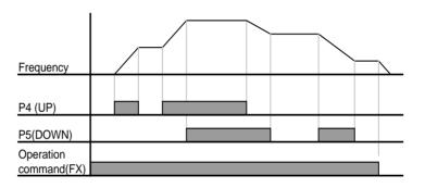
Up/down Save function: If P29, 'Save up/down frequency', is set to 1, the frequency before the inverter was stopped or decelerated is saved in P30.
