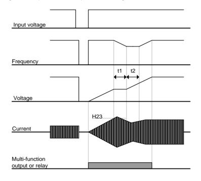
The followings show speed search operation during Instant Power Failure restart
