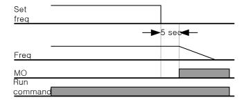
▶ Lost Preset F(I62=3): If the operating method(I62) is set as No. 3 Lost Preset in case of loss of the speed command, the protective action starts setting the frequency for continuance of operation.
