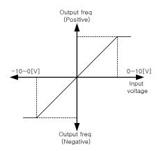
▶ I 2 ~ I 5: Setting input range and corresponding frequency to -10V ~ 0V V1 input voltage Ex) when minimum (-) input voltage is -2V with corresponding frequency 10Hz and Max voltage is -8V with run freq. 50Hz.
