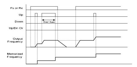
When F65 is 2: It is increased as many as step frequency set as F66 at the rising edge of multi-function input set as UP and if it is activated for 3 second, it operates like something set as "0". It is decreased as many as step frequency set as F66 at the rising edge of multi-function input set as DOWN and if it is activated for 3 second, it operates like something set as "0" and the accel/decel time is same with when stetted as "0".
