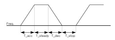
$$H76 = \frac{T\_dec}{T\_dec + T\_steady1 + T\_acc + T\_steady2} \times 100[\%]$$
