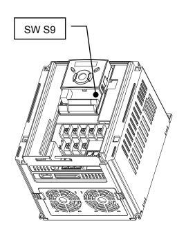
X Terminating Resistor applies to iG5A made after the latter half of 2013.
