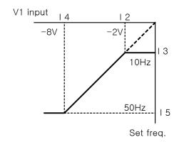
▶ 16 ~ I10: Setting input range and corresponding frequency to 0 ~ +10V V1 input voltage
