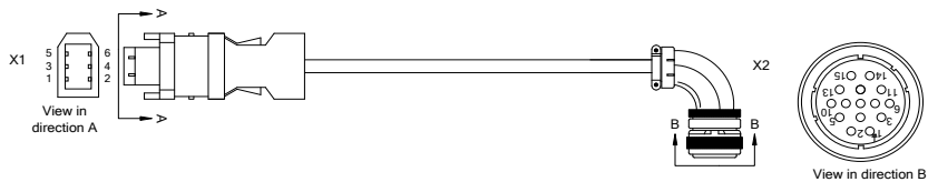
Figure 4-13 Absolute encoder motor wiring
